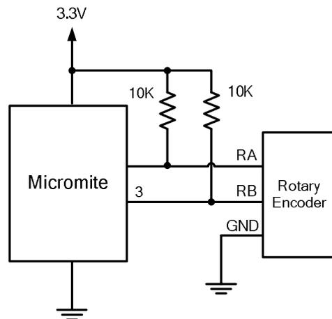
As the knob is turned the rotary encoder will generate a series of signals known as a Gray Code. The program fragment below uses an interrupt to detect and decode the code and update the variable `Nbr` accordingly.
