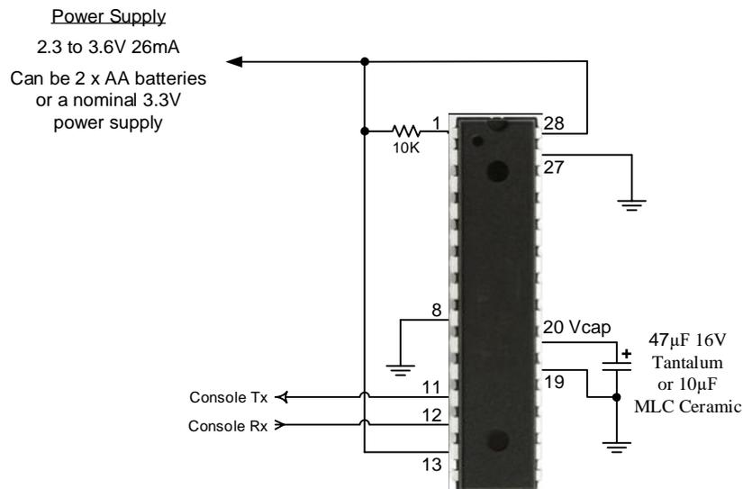
The PIC32 uses a high performance processing core and it can be susceptible to noise on its power supply. For this reason you should use a stable supply that you can trust.
