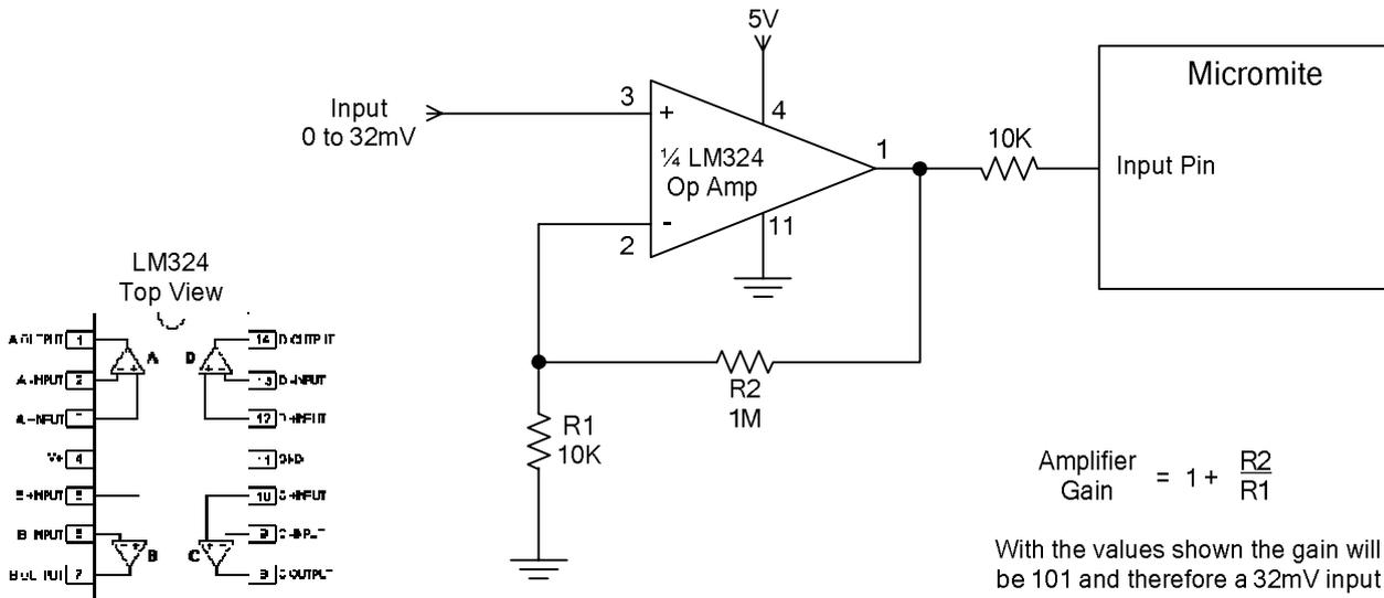
The gain of the amplifier is determined by the ratio of R2 to R1 plus 1 and using the components shown the gain is 101. This number should be used in the BASIC program so that the readings are scaled to represent the input voltage.
